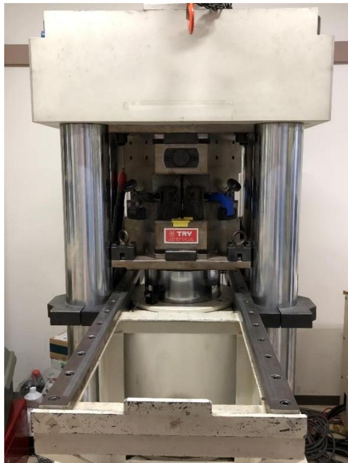
Fig. 2.2 700-ton hydraulic press of cubic high-pressure synthesis apparatus. (TRY ENGINEERING Co., Ltd.)
