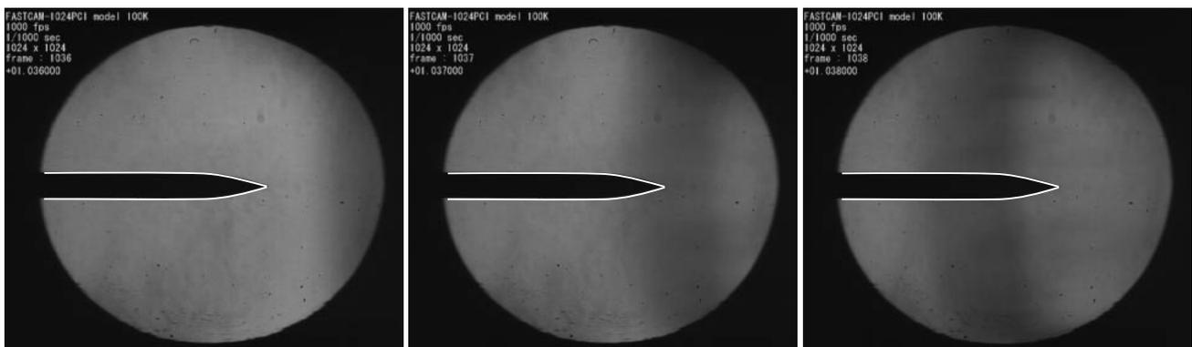
Fig. 7. Behavior of reflected compression wave for Mach 3 condition ( $t = 1.036\text{--}1.038\text{ s}$ ).
