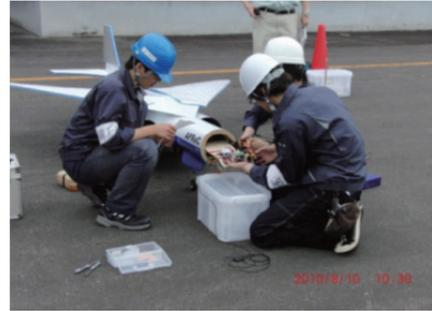
Fig. 14. Preflight check on onboard avionics.
