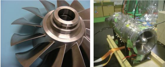
Fig. 11. The fabricated first-stage fan in the prototype counter-rotating axial fan turbojet (CRAFT) engine and its ground test facility.
