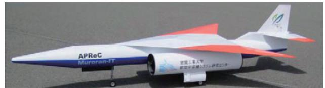
(b) The painted and fully equipped vehicle (without a Pitot boom).
