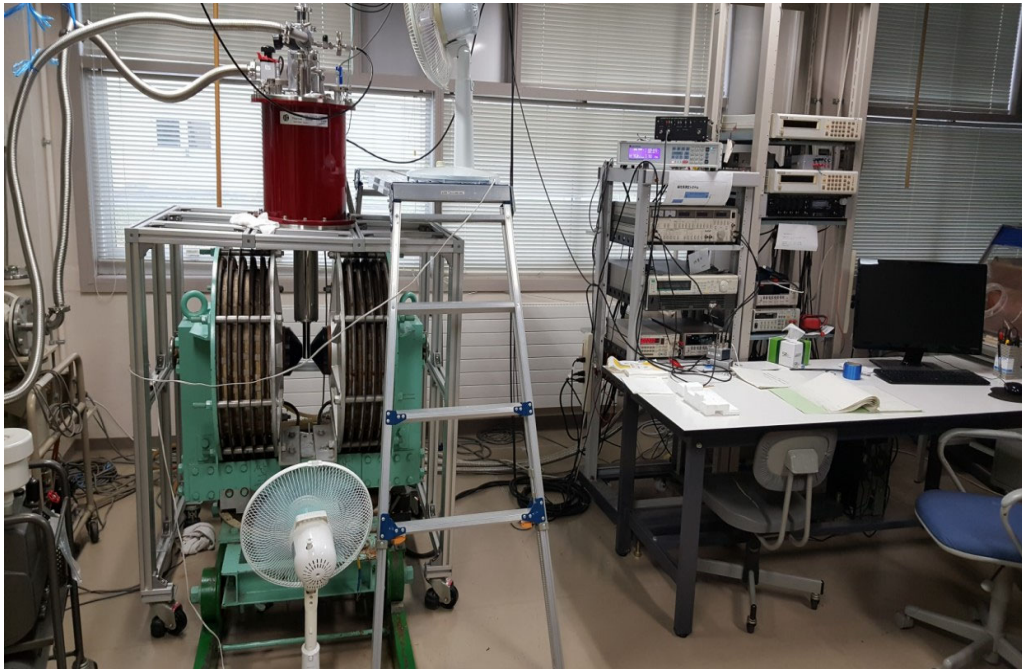
Figure 2.6 Electrical resistivity measurement system by laboratory-built
