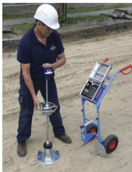
Figure 4.8 Portable Falling Weight Deflectometer (PFWD) apparatus
