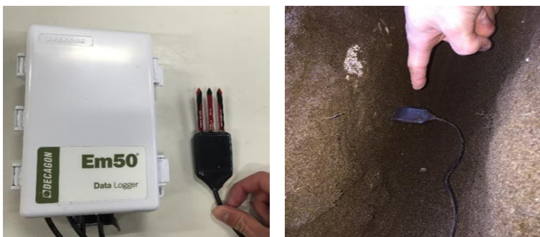
Figure 3.14 Temperature sensor installed in the excavation hole
