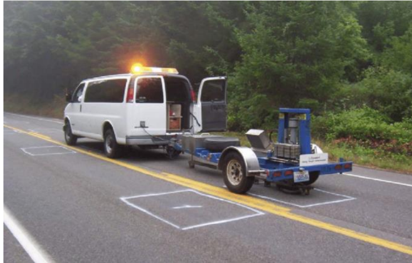
Figure 4.7 Falling Weight Deflectometer (FWD) apparatus
