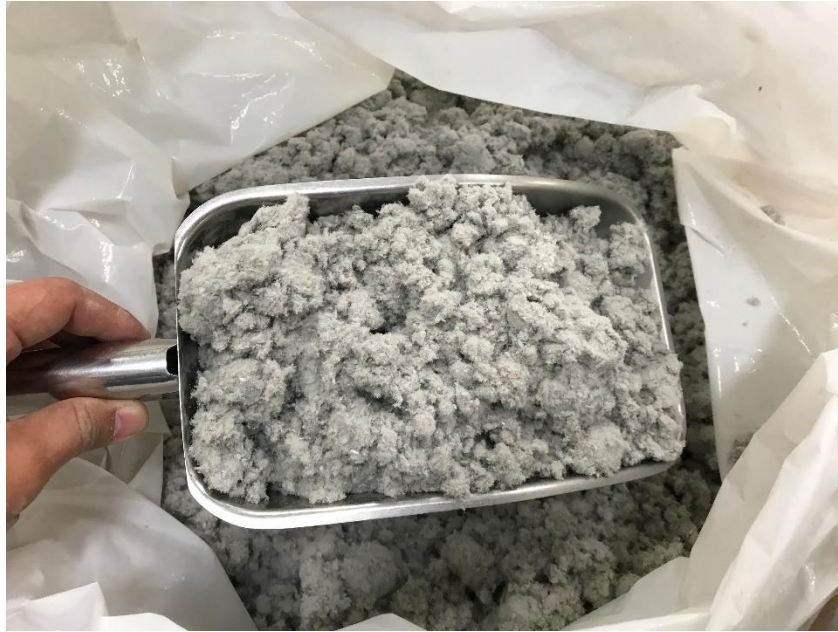
Figure 2.2 Fiber material was made by the newspaper
