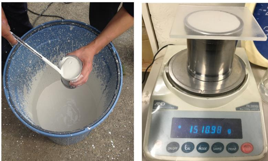
Figure 3.7 The density of the mixture was checked by AE mortar container
