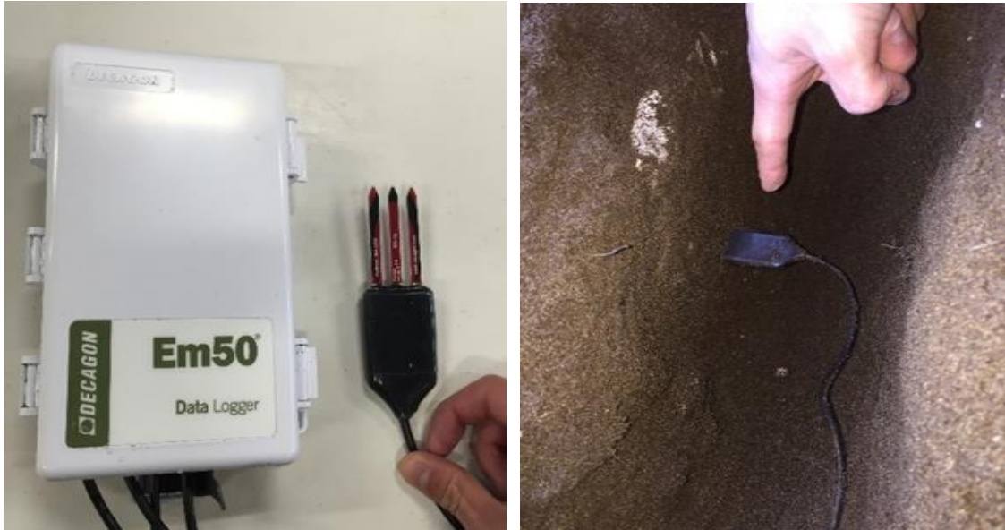
Figure 5.2 Setting temperature sensor in the model ground
