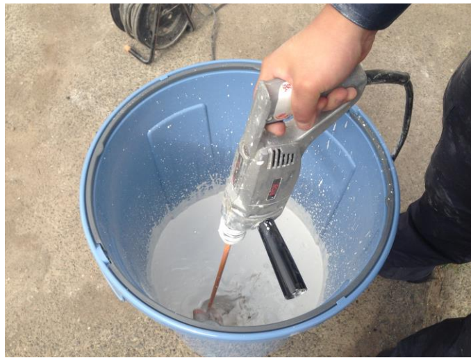
Figure 3.6 NSF-Clay and water were mixed in the bucket by hand mixer
