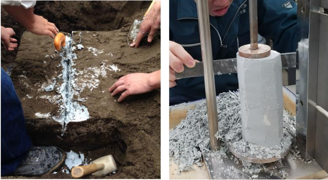
Figure 3.15 The samples prepared by trimming LSS retrieved from the test field
