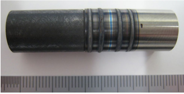
FIGURE 5 Photograph of Zircaloy-SiC/SiC composite joints with Wide Hook Slit 1 after fiber laser irradiation
