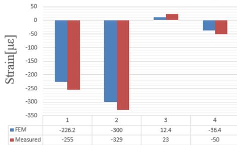
(b) Comparison of strains ① to ④ for Sequence 2
