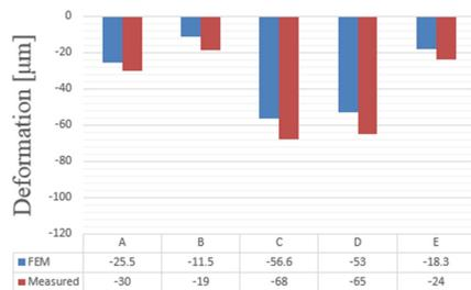
(a) Comparison of deformations A to E for Sequence 1
