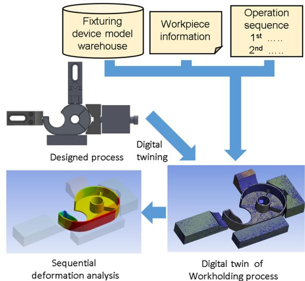
(b) Digital twinned workholding simulation
