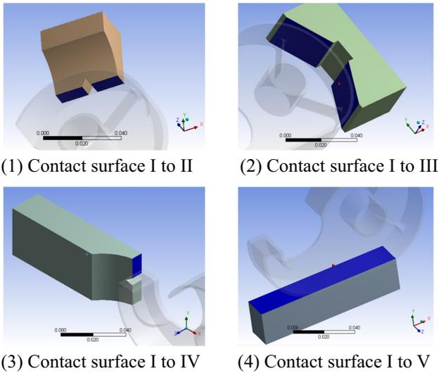
**Fig. 8.** Contact surfaces of workpiece and workholding instruments.
