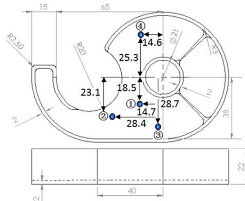
Fig. 6. Location of strain measurement points.
