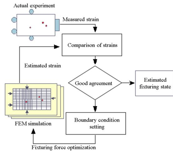
Fig. 2. Estimation flow of simple workholding state.
