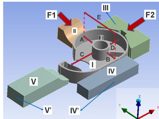
Fig. 7. Workholding setup and deformation measured position.
