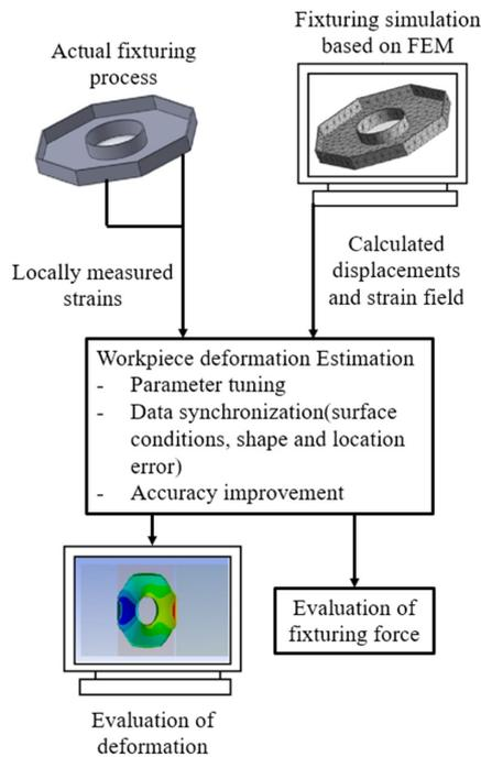
Fig. 1. Framework for on-machine estimation.
