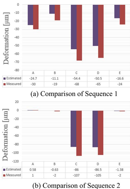
Fig. 13. Comparison of deformations (estimated and measured).
