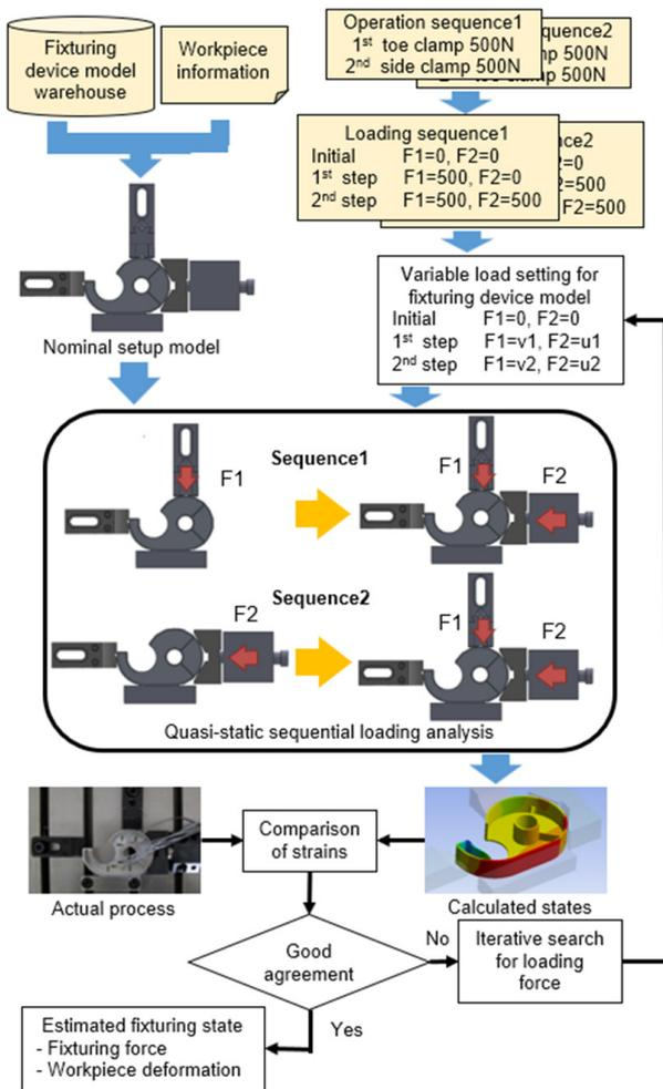
Fig. 4. Estimation flow of complex workholding state.
