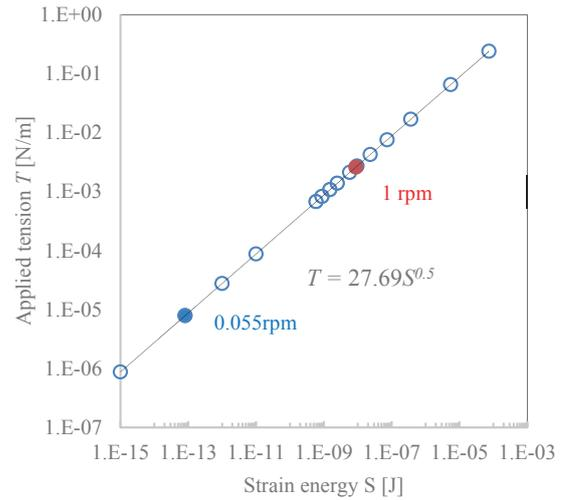
Fig. 15. Tension level versus strain energy for the estimation of equivalent tension.
