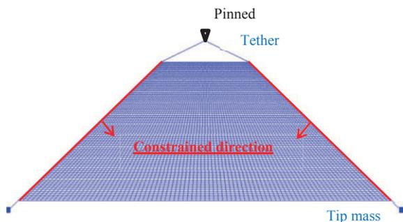
Fig. 14. FE model of sail membrane applied spin centrifugal force.
