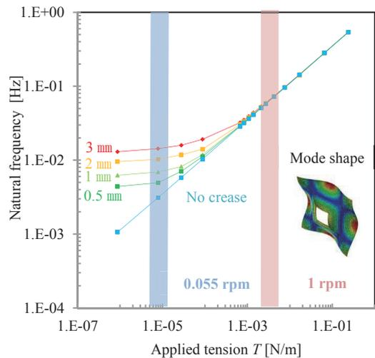
Fig. 13. Comparison of creased and flat membrane by natural frequency (similar mode shape is selected).
