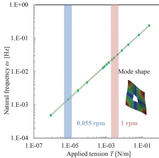
Fig. 11. Comparison of creased and flat membrane by natural frequency (mode1).
