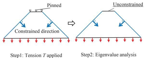
Fig. 9. Boundary conditions in each analysis step.
