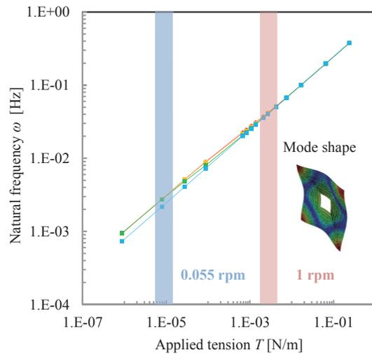
Fig. 12. Comparison of creased and flat membrane by natural frequency (mode 2).
