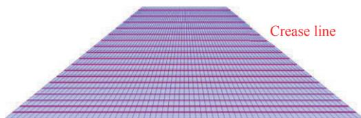
Fig. 10. FE model of solar sail membrane.
