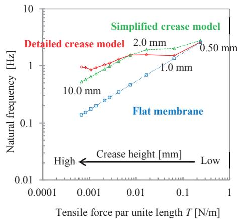
Fig. 6. Comparison of natural frequency among the three models.
