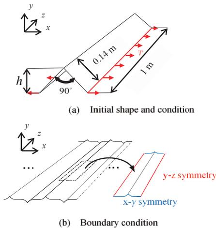
Fig. 2. Detailed model of a creased rectangular membrane.
