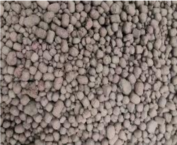
Fig. 2.3 The artificial lightweight coarse aggregate
