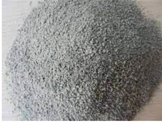
**Fig. 1.5** EPS bead mixture
