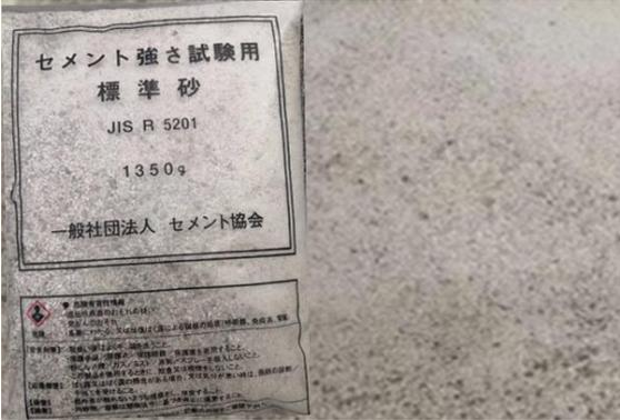
**Fig. 2.1** Cement standard sand
