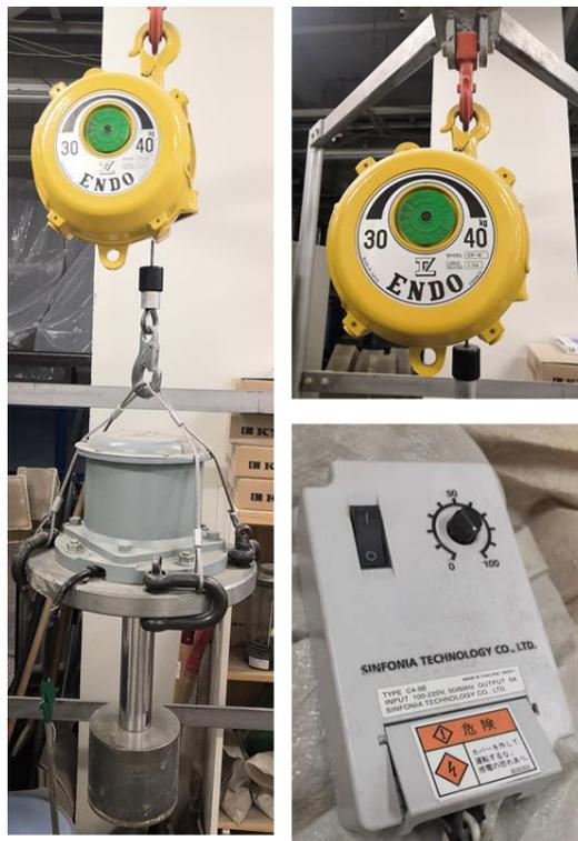
**Fig. 2.21** Top-loading vibrator apparatus
