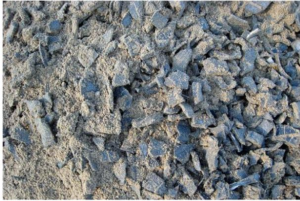
**Fig. 1.7** Rubber-soil mixtures
