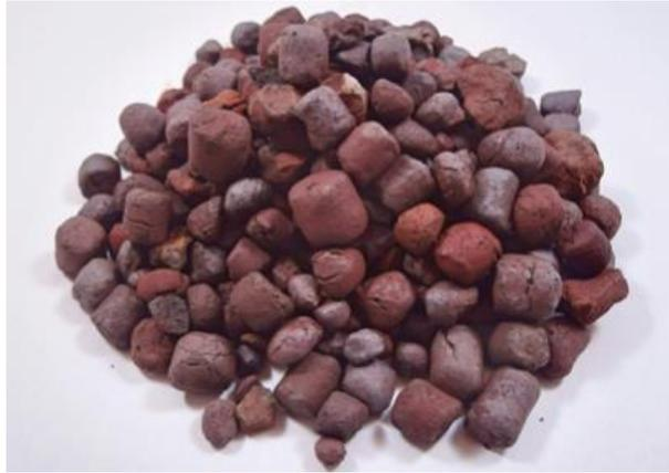
**Fig. 1.8** Lightweight aggregates
