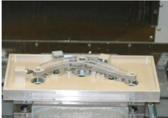
Fig.2-2 PAW fixture and bracket casting mounted in the vise for the Op #10 machining processes [36]
