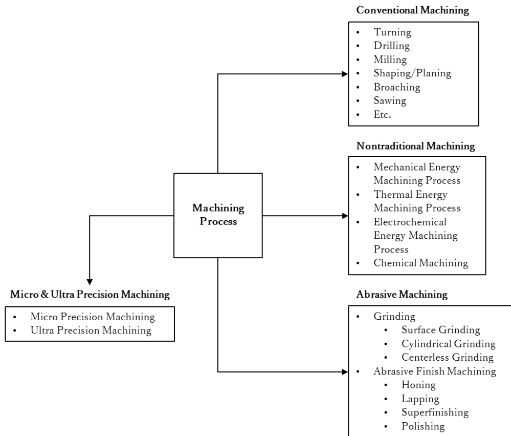
Fig. 2-1 Machining process classification
