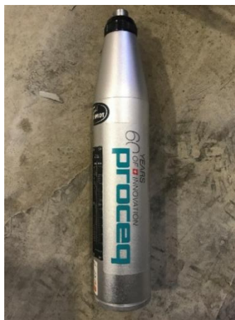
Fig. 3.6 N-type rebound hammer
