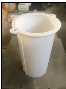
Fig. 3.4 \phi 100 \times 200 (mm) cylinder-type plastic mold
