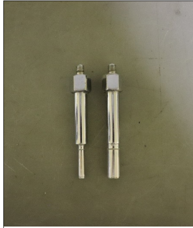
Fig. 5.3 Penetration needles (Left: cross-section 25 mm 2 , Right: cross-section 100 mm 2 )
