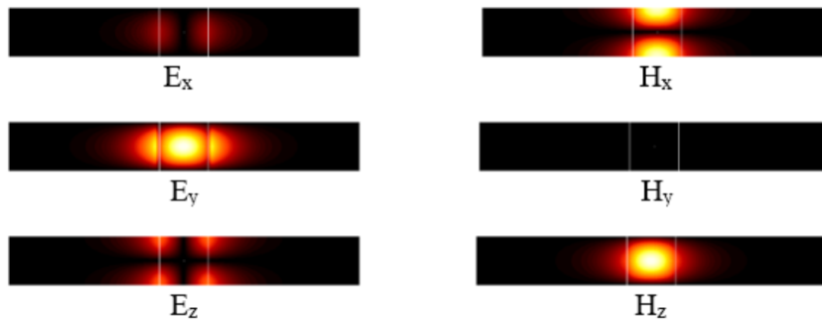
Figure 3.3: Field distribution of LSM_{01} mode at 60 GHz.
