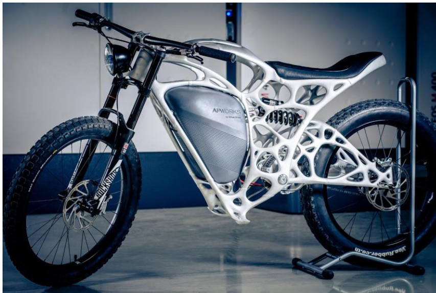
Fig. 1-1 The optimal design of bicycle body through topology optimization method (source: https://nlab.itmedia.co.jp/nl/articles/1605/22/news015.html )
