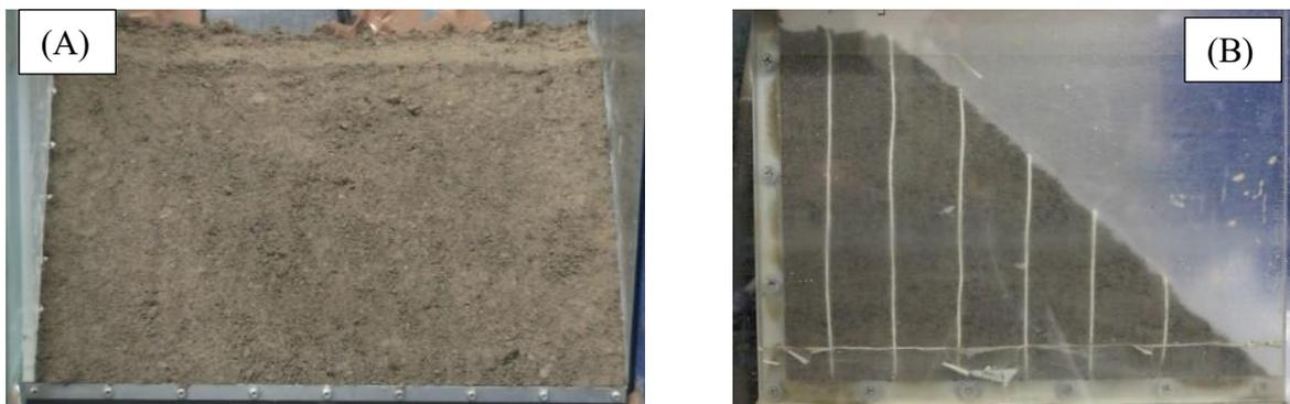
**Figure 3.10** The initial shape of the model embankments (A) front view (B) side view.
