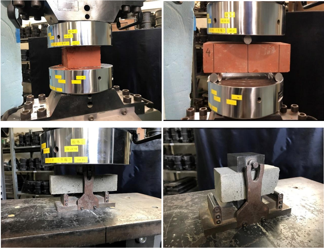
Figure 3.6. Compressive and flexural test for brick and mortar
