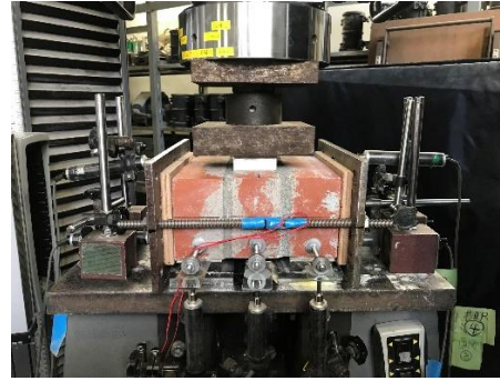
(b) Laying specimens on the machine
