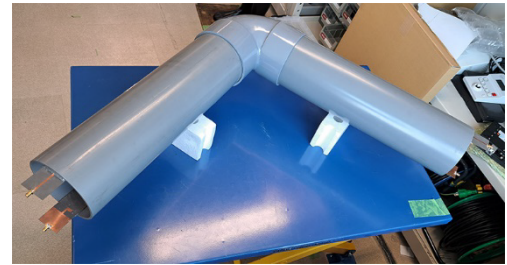
Fig. 15 Photograph of 1-m-long bent PVC pipe with which planar Yagi-Uda antennas are attached.
