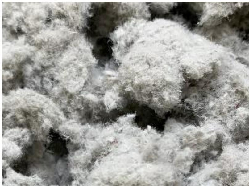
**Figure 2-2** Fiber material made by pulverized newspaper
