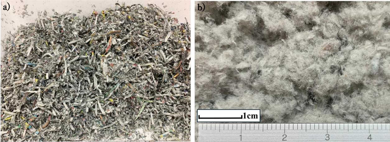
**Figure 3-1** a) Pulverized newspaper; b) Fiber material made by pulverized newspaper (with scale: cm)
