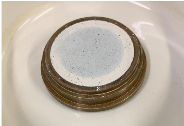
**Figure 3-4** Trimmed specimen
