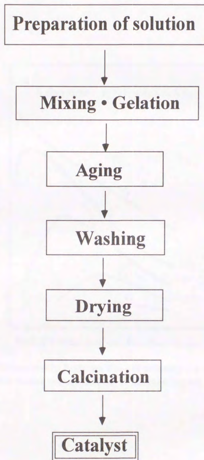
Fig.1-1 Schematic diagram of catalyst preparation process.
