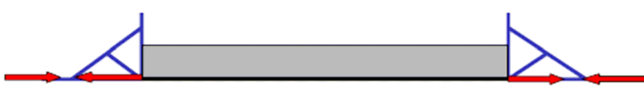
Fig.3.12 Prestressing the sheet by jacking directly to the strengthened beam itself.
