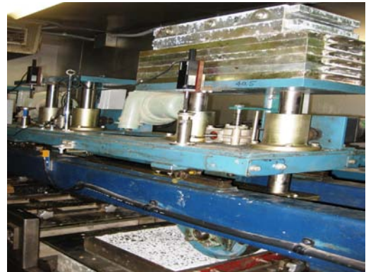
Photo 8.3: Special loading of Wheel tracking test
