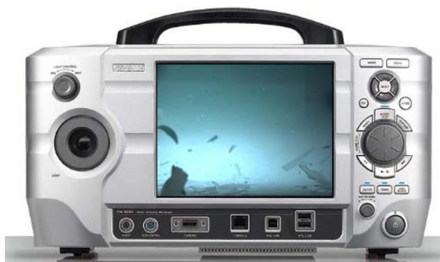
Figure 2.6: The high speed video camera with a microscope (KEYENCE VW-6000 Lens VW-Z2)
