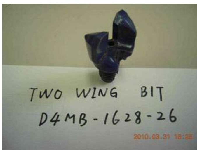
Figure 2.7: The Two-Wing bit (D4MB-1628-26, by Sandvik Mining and Construction)
