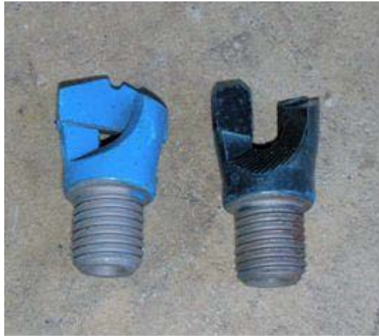
Figure 5.2: Bits used in this experiment ( \Phi 27 mm, Left: Spade; Right Two Wing).
