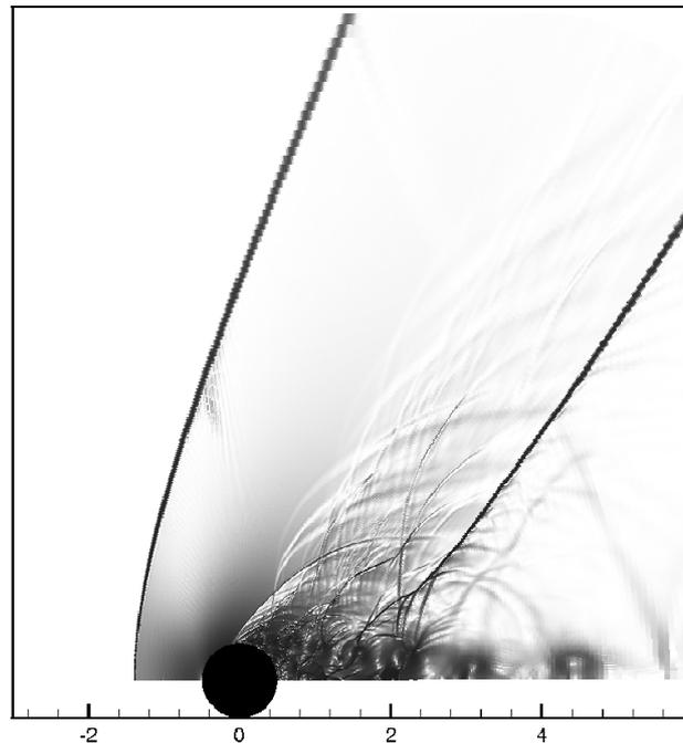
図 7.5. Pressure distribution around a sphere flying with  $Ms = 1.13$ : Distance scale normalized by model diameter.
