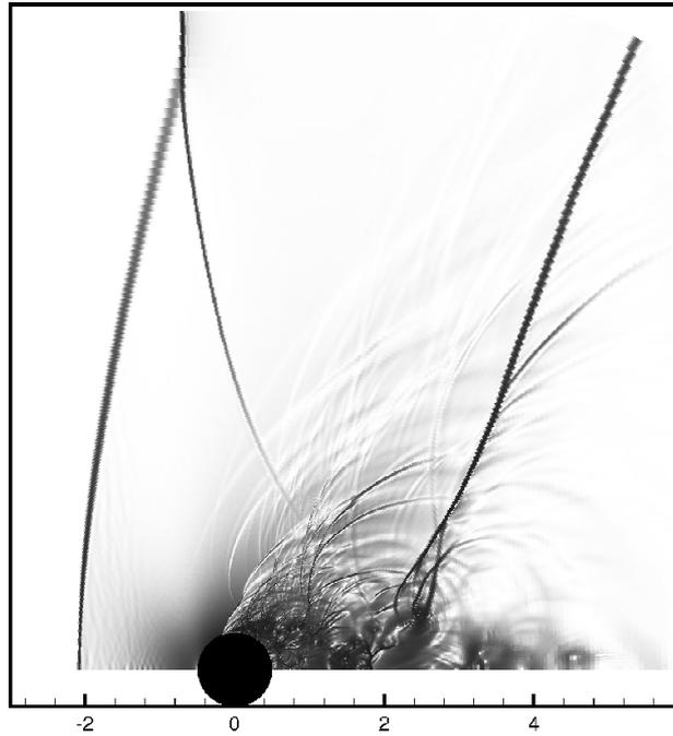
図 7.7. Pressure field around a decelerating sphere:  $M = 1.04$ .
