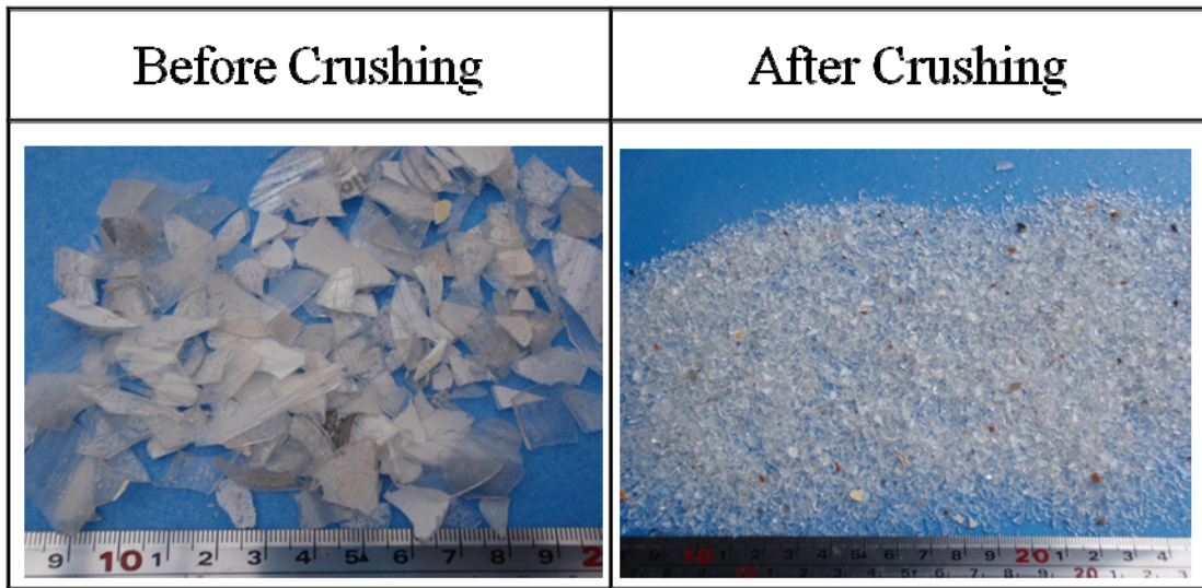
Fig. 4-4 Crushed glass of waste fluorescent lamp.
