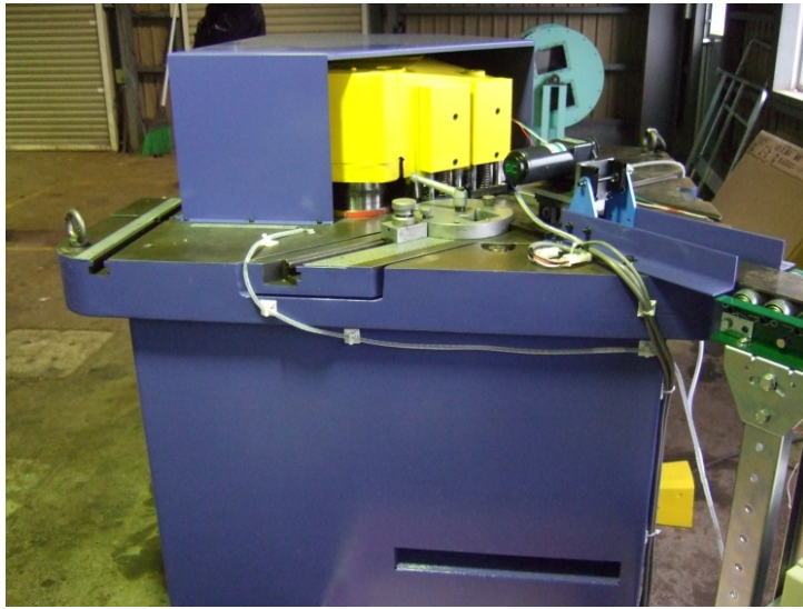
Fig. 5-4 Photos of guillotine cutting testing machine.
