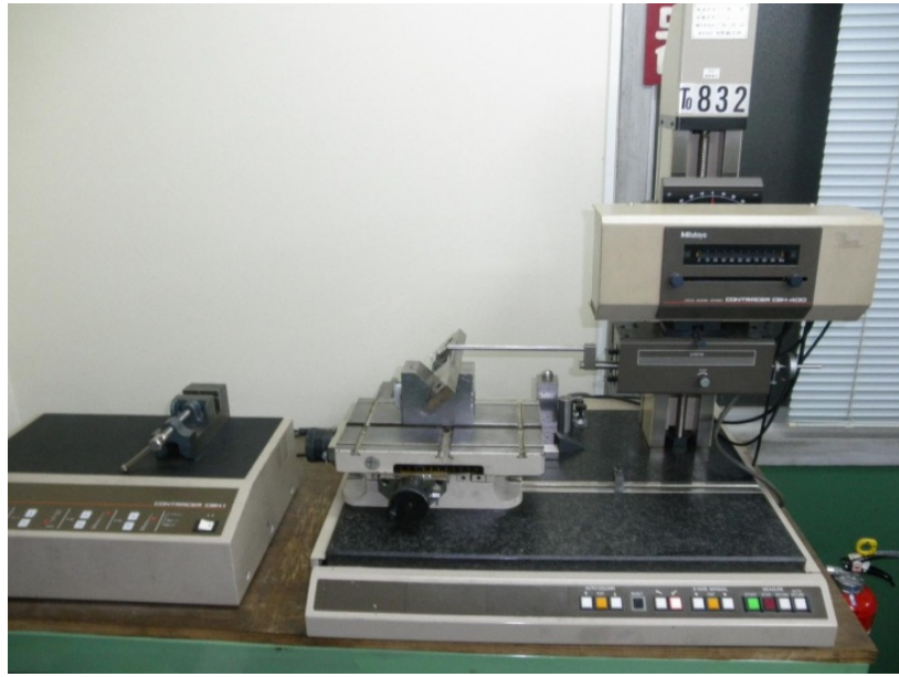
Fig. 5-12 Photo of shape measuring device.
