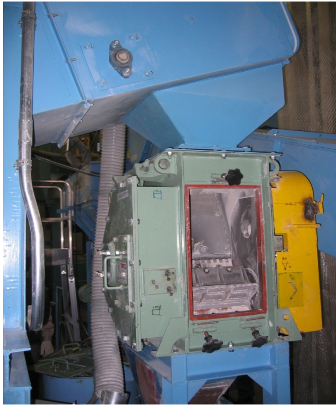
Fig. 4-3 Uniaxial rotational glass shredder.
