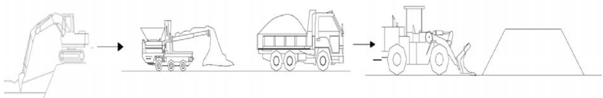
Figure 2.7 Two stages construction method using lightly lime/cement treated clayey soils (Hino et al., 2008)
