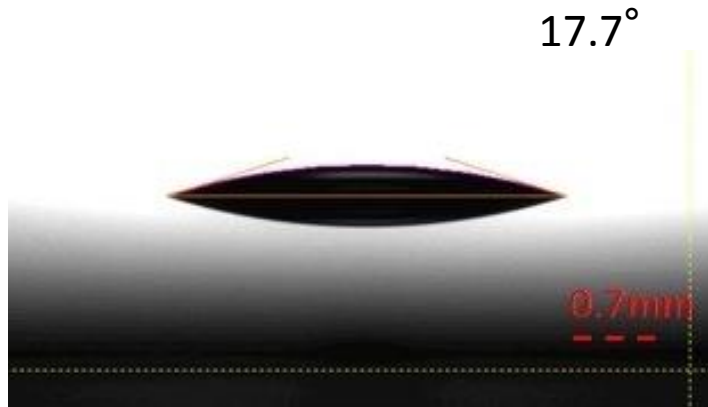
図 2.12(a) 親水面(水晶面)の純水の接触角写真 Fig.2.12(a) Photograph of contact angle of hydrophilic surface. (Pure water 1 \mu L).
