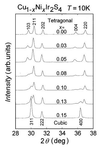
FIG. 8. X-ray diffraction pattern for  $0.00 \le x \le 0.15$  at 10 K over the angle range of  $28 \le 2\theta \le 38^\circ$ .
