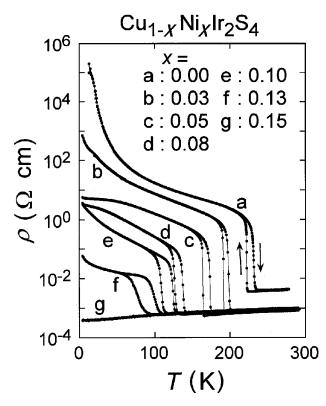
FIG. 2. Temperature dependence of electrical resistivity  $\rho$  for sintered specimens Cu<sub>1-x</sub>Ni<sub>x</sub>Ir<sub>2</sub>S<sub>4</sub> for  $0.00 \le x \le 0.15$ .
