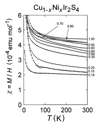
FIG. 5. Magnetic susceptibility vs temperature of  $Cu_{1-x}Ni_xIr_2S_4$  for  $0.15 \le x \le 1.00$ . The applied magnetic field is 10.000 kOe.
