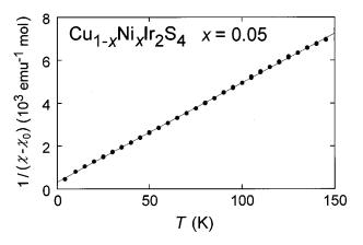
FIG. 9. Temperature dependence of the inverse susceptibility  $(\chi - \chi_0)^{-1} = (M/H)^{-1}$  for x = 0.05.
