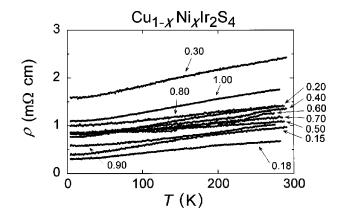
FIG. 3. Temperature dependence of electrical resistivity  $\rho$  for sintered specimens Cu<sub>1-x</sub>Ni<sub>x</sub>Ir<sub>2</sub>S<sub>4</sub> for  $0.15 \le x \le 1.00$ .
