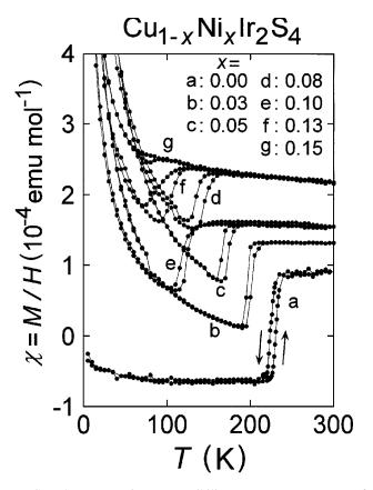
FIG. 4. Magnetic susceptibility vs temperature of  $Cu_{1-x}Ni_xIr_2S_4$  for  $0.00 \le x \le 0.15$ . The applied magnetic field is 10.000 kOe.
