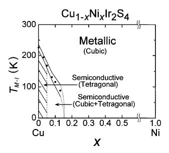
FIG. 10. A phase diagram of  $Cu_{1-x}Ni_xIr_2S_4$  for temperature vs concentration x. The solid circles indicate the *M-I* transition temperature  $T_{M-I}$ . Two solid curves show the width of the temperature hysteresis for the *M-I* transition, which corresponds fairly well to the structural transformation; see the text.
