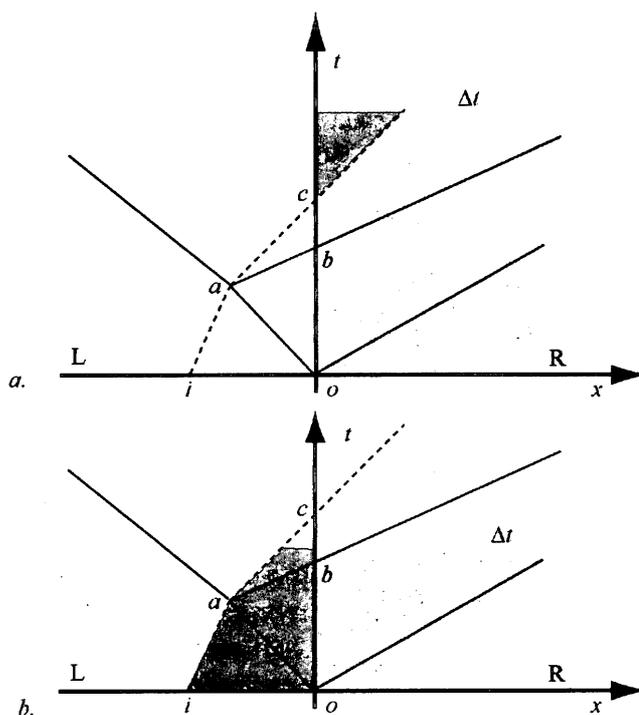
Fig. 1 Wave system for the Riemann solver
