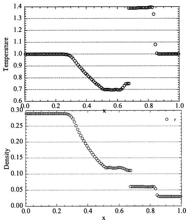
Fig. 2 Numerical result of a shock tube problem
