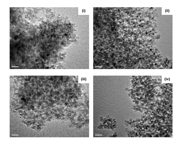
Fig. 8 TEM images of NM-P/SiO $_2$  catalysts reduced at 500 °C. (i) Rh-P, (ii) Pd-P, (iii) Ru-P, and (iv) Pt-P.
