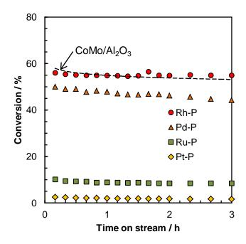
Fig. 4 Hydrodesulfurization of thiophene over NM-P/SiO  $_2$  catalysts reduced at 550  $^{\circ}\text{C}.$
