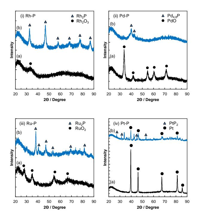
Fig. 3 XRD patterns of NM-P/SiO<sub>2</sub> catalysts after (a) calcination at 500 °C and (b) TPR measurement. (i) Rh-P, (ii) Pd-P, (iii) Ru-P, and (iv) Pt-P.
