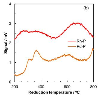
Fig. 2 TPR spectra of calcined NM-P/SiO $_2$  catalysts. (a) TPR spectra of NM-P catalysts, (b) Magnified TPR spectra of Rh-P and Pd-P catalysts from 200 to 800 °C.
