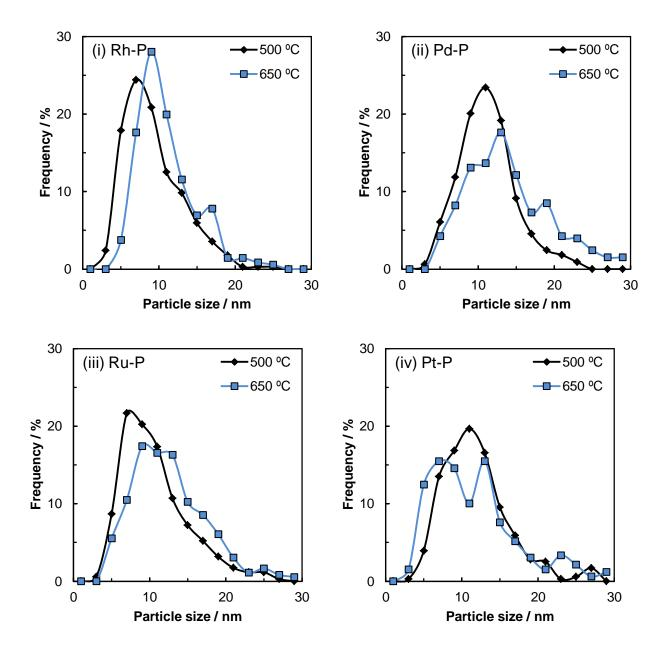
Fig. 9 Particle size distributions of NM and  $NM_XP_Y$  in  $NM-P/SiO_2$  catalysts reduced at 500 and 650 °C. (i) Rh-P, (ii) Pd-P, (iii) Ru-P, and (iv) Pt-P.
