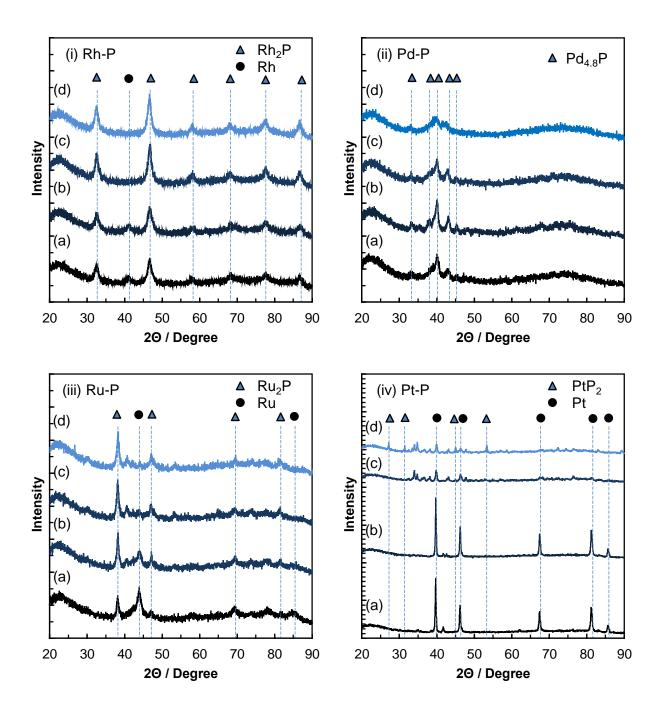
Fig. 7 XRD patterns of NM-P/SiO<sub>2</sub> catalysts after reduction at (a) 500 °C, (b)  $^{\circ}$ C, (c) 600 °C, and (d) 650 °C. (i) Rh-P, (ii) Pd-P, (iii) Ru-P, and (iv) Pt-P.
