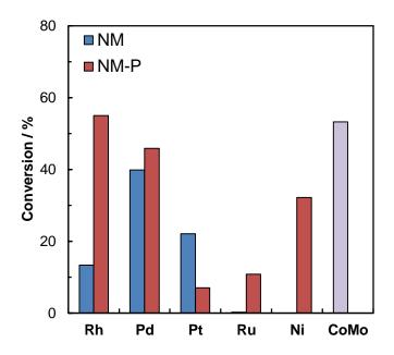
Fig. 6 HDS activities of  $NM/SiO_2$  and  $NM-P/SiO_2$  catalysts. Reduction temperature: 350 °C (Pd), 400 °C (Pt, Ru), 450 °C (Rh), 500 °C (Pd-P, Pt-P), 550 °C (Rh-P), 650 °C (Ru-P, Ni-P).
