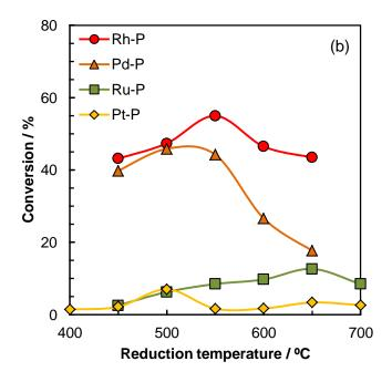
Fig. 5 Effect of reduction temperature on HDS activities of (a) NM/SiO  $_2$  and (b) NM-P/SiO  $_2$  catalysts.
