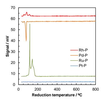
Fig. 1 TPR spectra of calcined  $NM/SiO_2$  catalysts.
