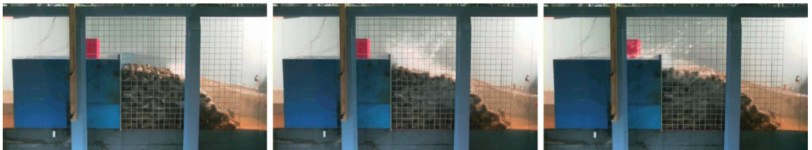
写真-3 越波状況 ( T_{1/3}=11.0s, H_o'=3.0m )
