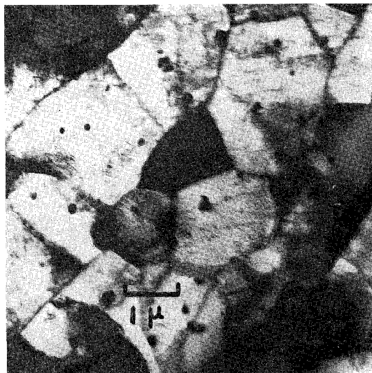
Photo 9. Transmission electron micrograph near the crack by thermal fatigue after 300 cycles. specimen and thermal cycle: same as Photo. 8.
