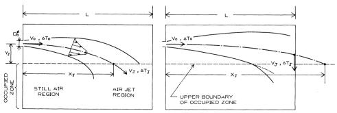
Fig.2 Schematic flow pattern in summer cooling
