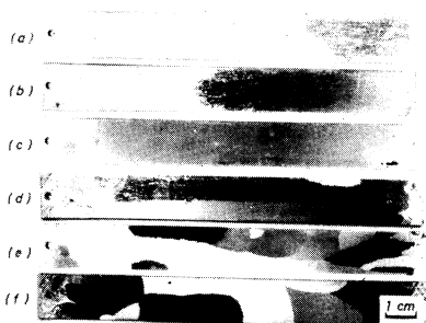
Fig. 5 Growing grains by strain-annealing process in the temperature-gradient furnace at the inserting velocity of 10 mm/h. Pre-annealed for 2h at 400°C and then strained to (a) 0%, (b) 1%, (c) 2.5%, (d) 3.5%, (e) 4% and (f) 5%. Left-hand of specimens is low temperature side.
