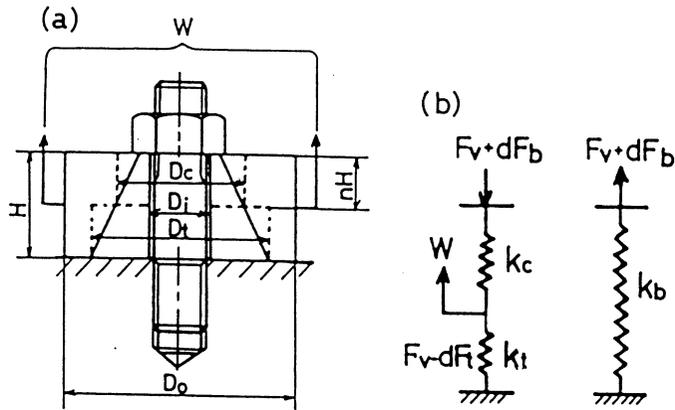
Fig.3 Stud bolted joint and spring elements model
