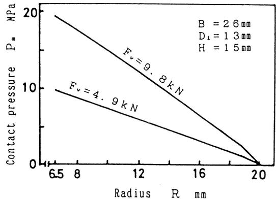
Fig. 6 Relation between contact pressure radius against preload
