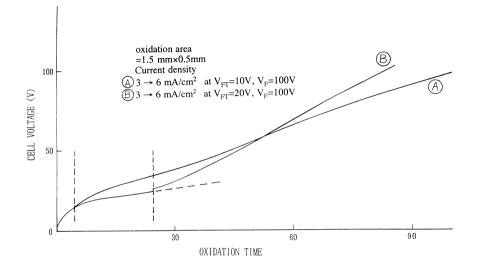
Figure 2 Cell voltage versus anodization time for two cases of small-area constant current anodization.
