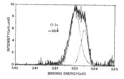
Figure 10 XPS O Is spectra of the 30 ÅSi anodic oxide film.
