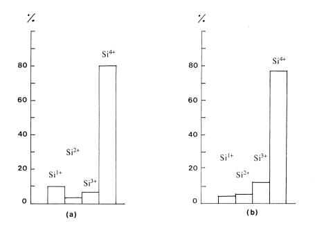
Figure 16 Si atoms having different valence states in the composition of Si-SiO<sub>2</sub> interface oxide of about 30 Å. (a) small-area anodic oxide, (b) large-area anodic oxide.
