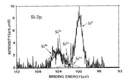
Figure 13 XPS Si 2p spectrum appeared form the 30 Å Small-area anodic oxide film.
