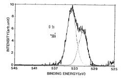
Figure 9 XPS Is spectra is separated into its component spectrum. Sample was small-area Si anodic oxide film.
