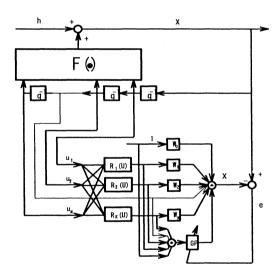
Fig. 2. Nonlinear time series identification system
