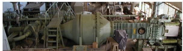
Fig. 8. Outline configuration of the indoor components of the supersonic wind tunnel at the former Institute of Space and Aeronautical Science, University of Tokyo.
