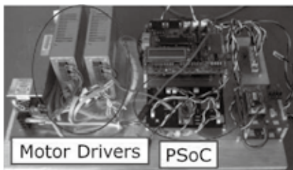
Fig.6 Electrical device for the steering control
