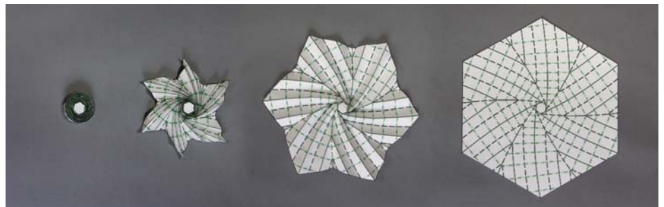
(b) Deployment sequence of an origami model with modified spiral folding
