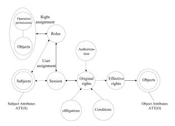
FIGURE 5. Role-based usage control for access.
