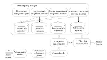
FIGURE 8. Access flow and usage control system components.
