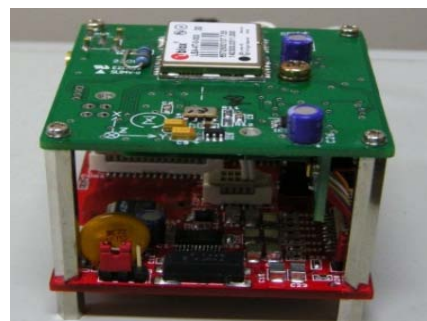
Fig. 1 Overview of the present navigation avionics.
