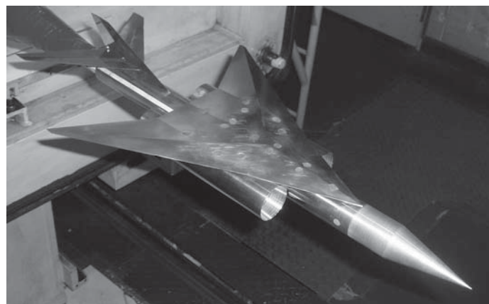
Fig. 2. Wind-tunnel test at JAXA/ISAS using the M2006 model.
