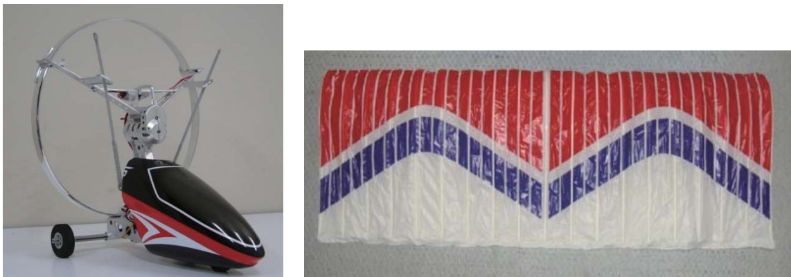
Fig.2 The fuselage and the canopy of the parafoil experimental vehicle.
