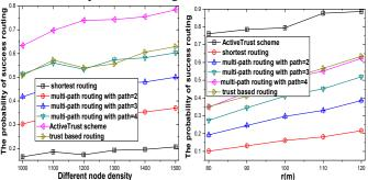
Fig. 32. The probability of successful routing under different nodal densities
