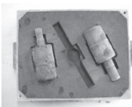
Fig. 4 Frozen mold and frozen core
