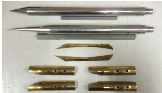
(c) Area rule modification parts.
