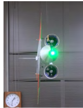
Fig. 4.2. Measurement of moment of inertia around the y-axis.
