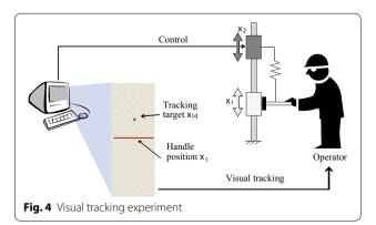
The actuator's position,  $x_2$ , is synchronized with the operator's motion by means of a periodic input control. Moreover, the actuator has a phase difference  $\psi$  for skill assist control. The three ideal positions are thus described as
