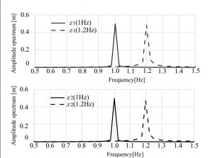
(b) Examples of the frequency entrainment characteristics of the controller
