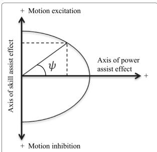
**Fig. 2** Concept image of the relation between the power assist effect and the skill assist effect
