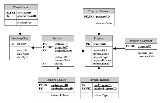
Figure 7: Ontology storage structure in relational database model.
