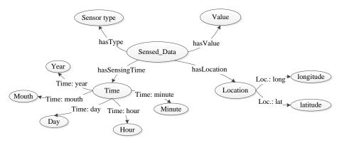
Figure 5: Description of heterogeneous data generated by experimental sensors.
