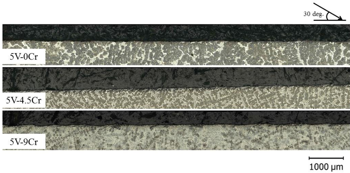
(a) Cross section observed along the impact direction
